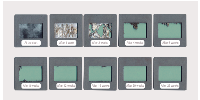
The slides show the disintegration of NatureFlex NM under ambient conditions. After 4 to 6 weeks, the film has essentially disappeared.
